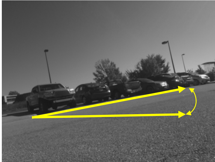
Figure 1.8 Photo taken by the OpenCV software at 239 seconds into testing. Limitations in sensitivity lead to inaccurate vehicle identification. Example of bicycle sway and tilt shown.
