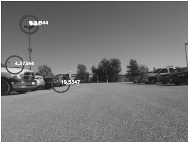
Figure 1.9 Photo taken by the OpenCV software at 201 seconds into testing. Not all objects identified OpenCV are vehicles.
